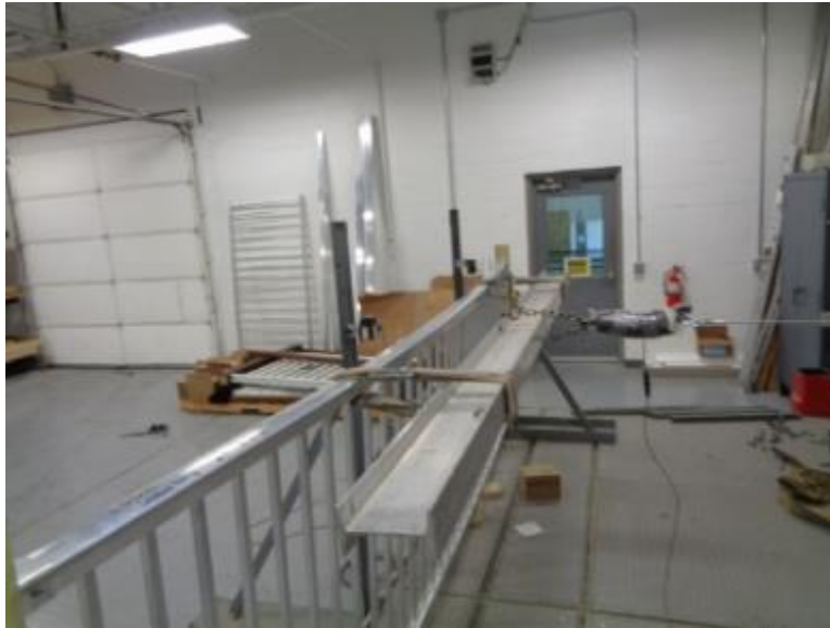
Photo No. 3 Uniform Horizontal Load on Top Rail
